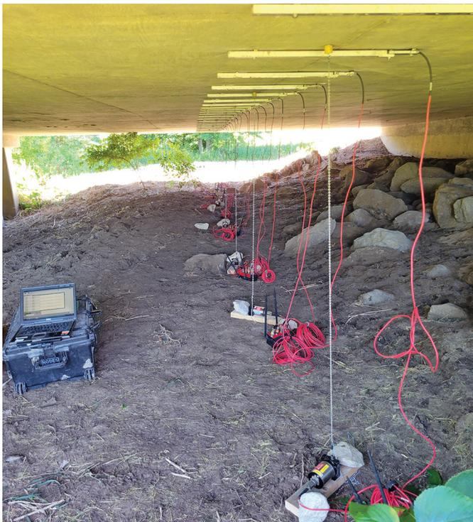
*Instrumentation of a bridge for live load testing*
