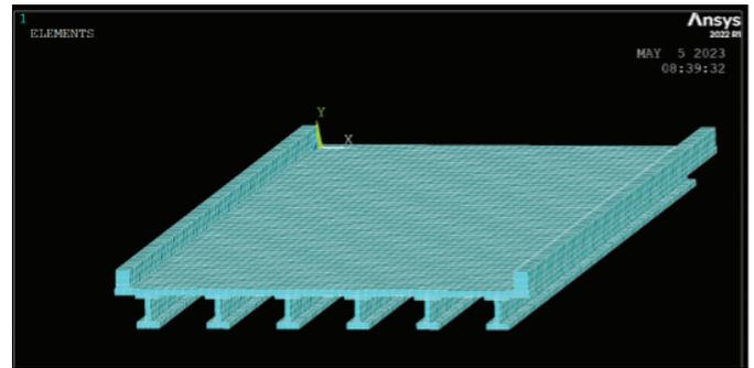
*Typical FE model of a PC bridge*
