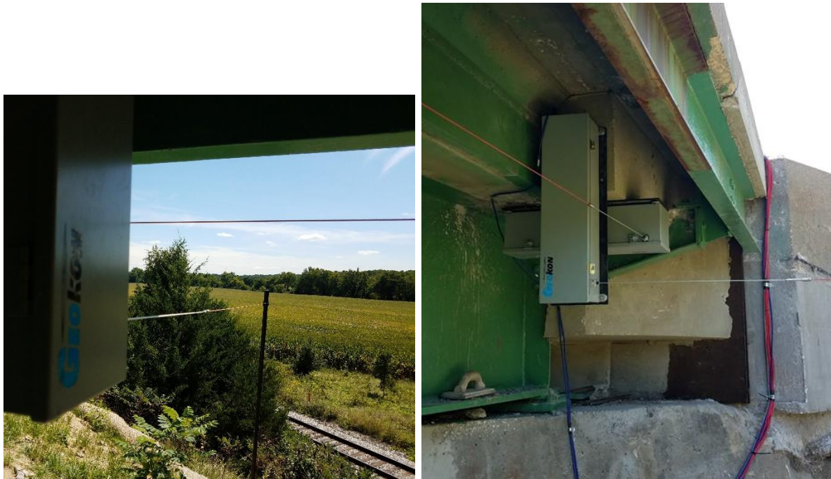
Figure 4.7. Jasper County 118—displacement transducer with reference post (left) and longitudinal and transverse displacement transducers attached at the acute bridge corner (right)
