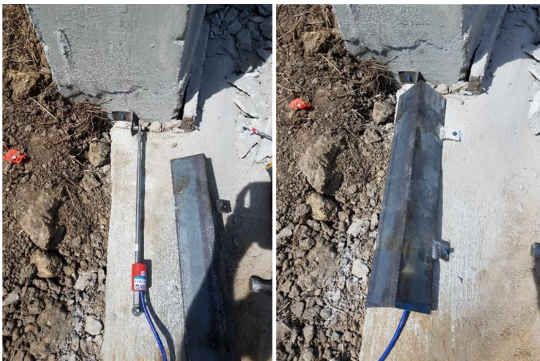
Figure 4.6. Jasper County 118—crackmeter without protective cover (left) and crackmeter with protective cover installed (right)
