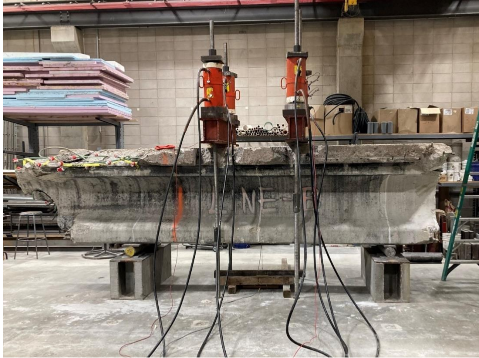
Figure 42. Girder end shear test configuration
