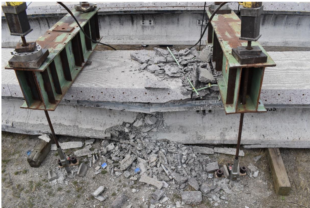
Figure 59. Girder E after failure at midspan
