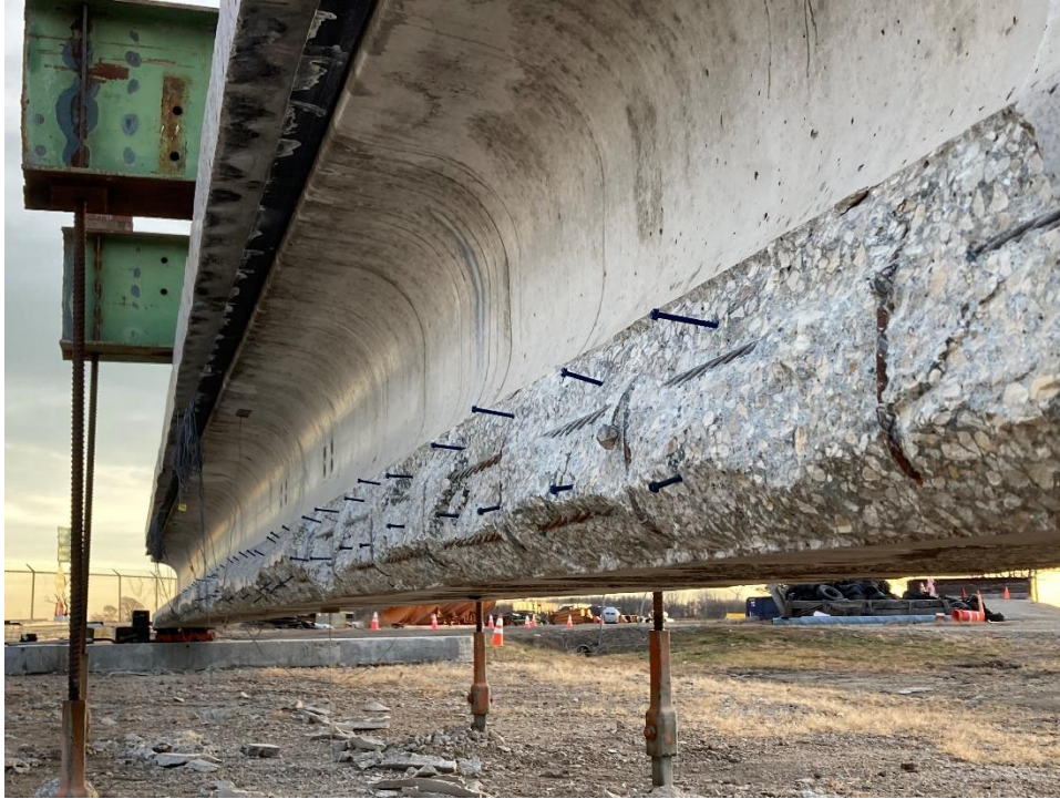
Figure 75. Concrete anchors into bottom flange
