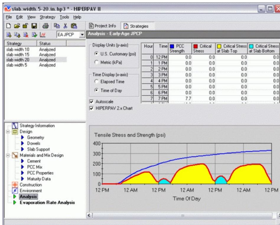
It should be noted that concrete can set up at different rates through the thickness of the slab. In late season paving, for example, the bottom of the slab (resting on warmer ground) may gain strength more rapidly than the top of the slab (exposed to cool air). In this case, sawing may need to begin sooner than would be suggested by the scratch test.
