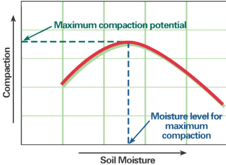
**b. Moisture-density curve for subgrade soil**
