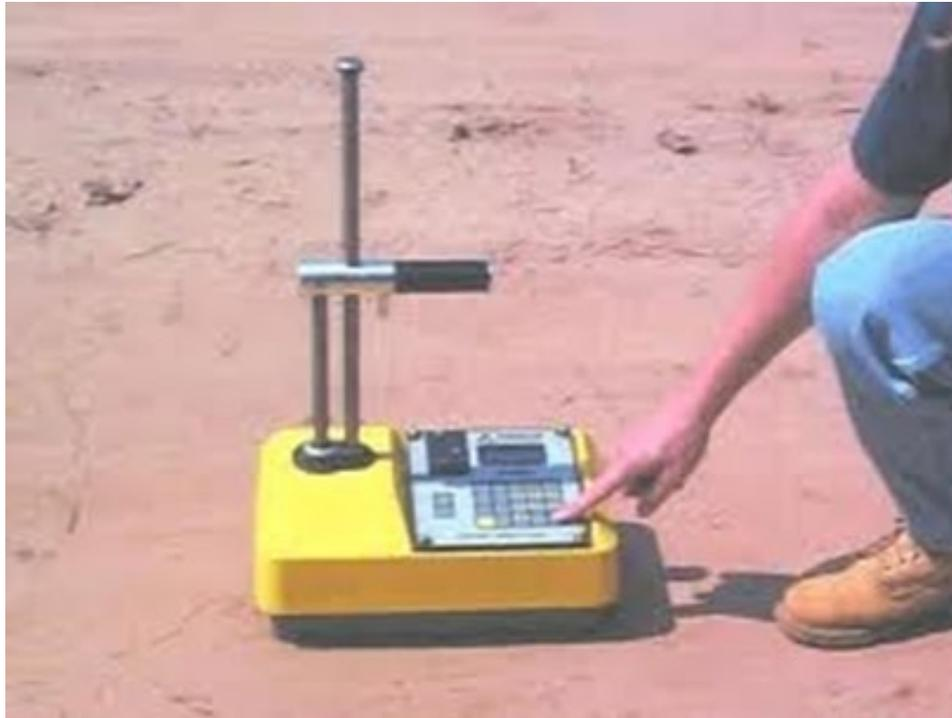
**a. Nuclear density gauge to determine in-place density**
