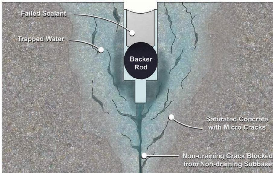
a. Poor joint sealant leading to saturation in concrete joint, resulting in micro cracking
