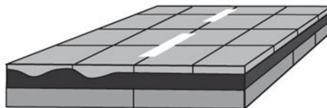
**b. Schematic of BCOA of a composite pavement**
