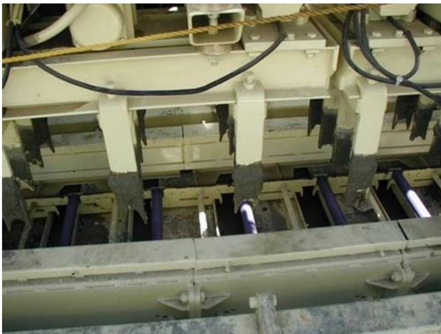
**b. Close-up of the dowel bar inserter on a paving machine**
