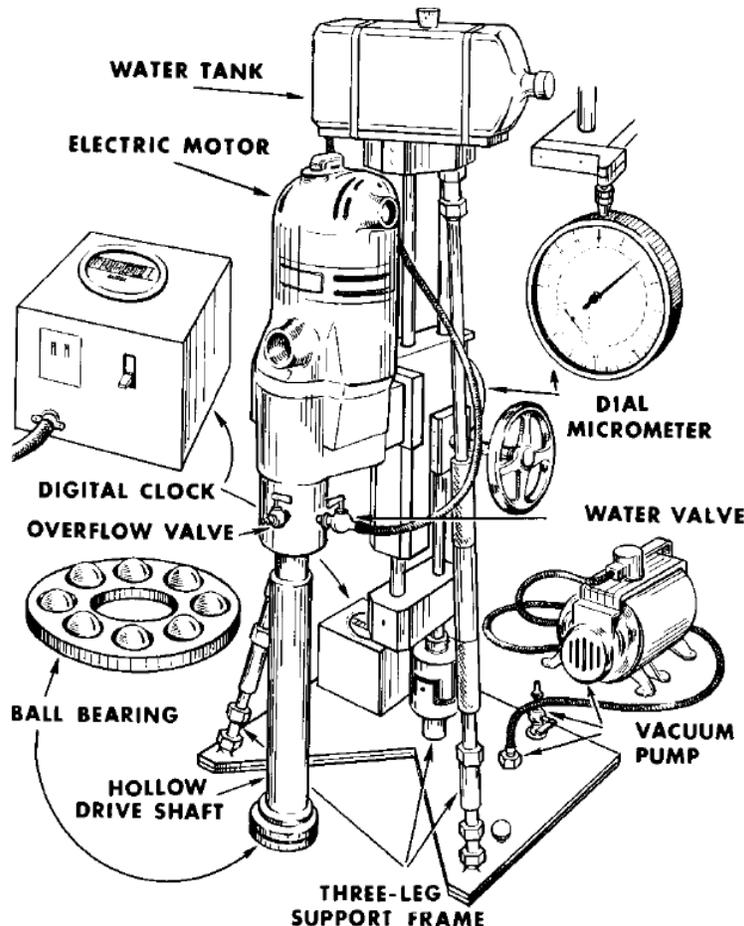
Reprinted, with permission, from *ASTM C779/C779M - 12 Standard Test Method for Abrasion Resistance of Horizontal Concrete Surfaces*, ©ASTM International; a copy of the complete standard may be obtained from ASTM International, <https://www.astm.org>
