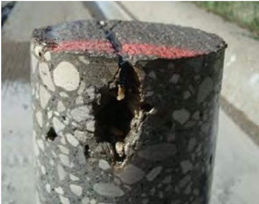
b. Longitudinal freeze damage from backer rod trapping water beneath sealant
