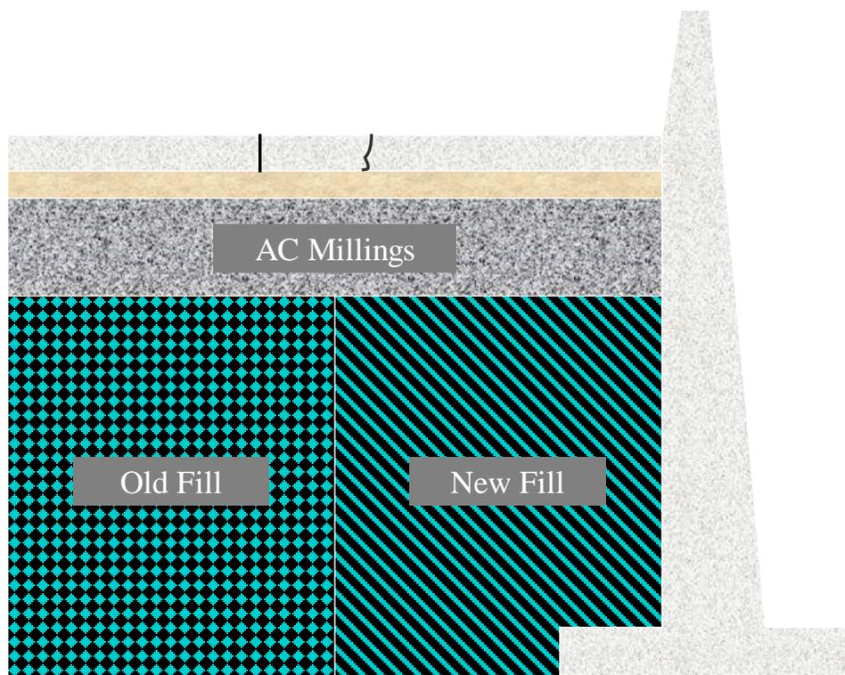
b. Cross-section of a fill section showing different fill material resulting in differential vertical movement resulting in longitudinal pavement cracking
