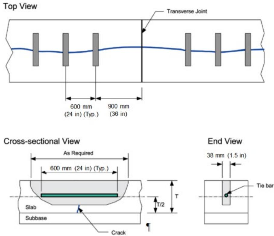
a. Schematic of slot stitching
