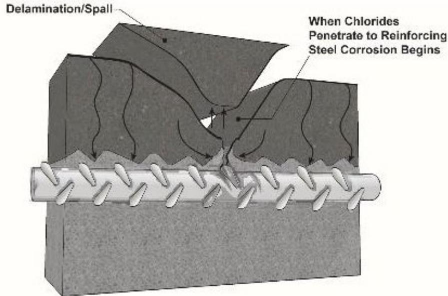
**a. Cross-section of concrete with a textured tie bar with some corrosion embedded in the concrete**
