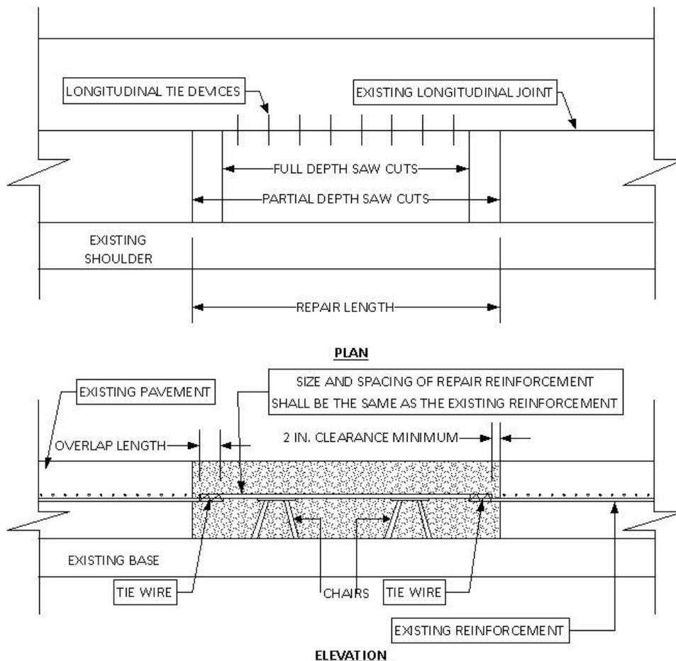
a. Schematic of CRCP full-depth repair
