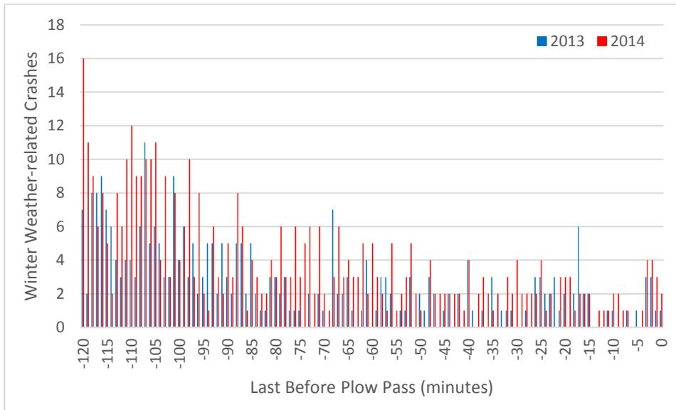
**Figure 20. Last before snowplow pass, crash time interval**
