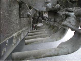
The image shows a close-up of the rollers on a paver, which are used to vibrate the concrete into the base.
