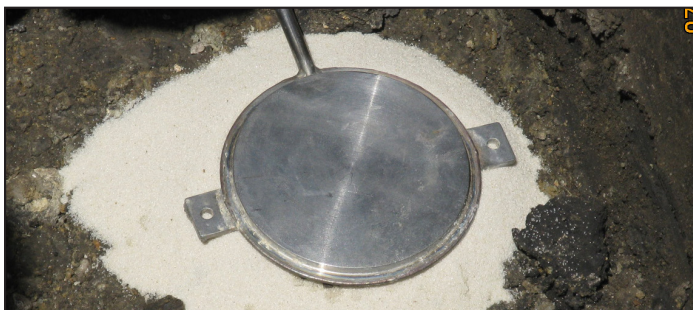
Figure 6. Piezo-electric earth pressure cell installed in subgrade layer
