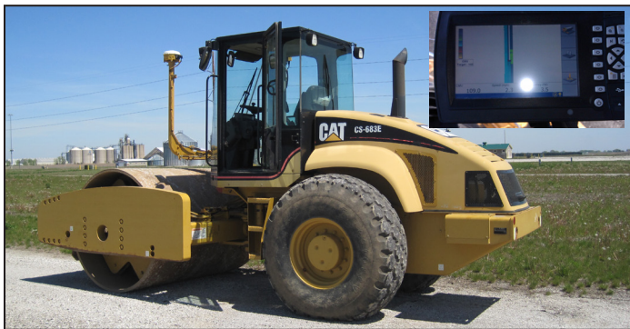
Figure 5. CS683 vibratory smooth drum roller with RICM system and on-board RICM system display (inset)
