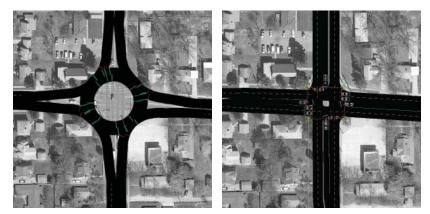
Models of two alternative improvement projects proposed for an intersection in Ames, Iowa: roundabout (left) and turning lanes (right)
