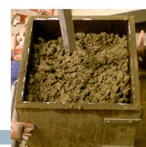
• A 1" diameter stinger vibrator is inserted into the center of the box over a three count and then removed over a three
