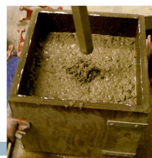
The sides of the box are then removed and inspected for honey combing or edge slumping
