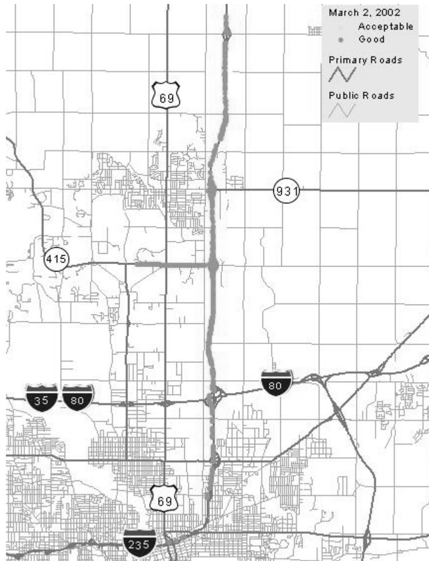
**Figure 18: Sample Peak Friction Measurements taken March 2, 2002**
