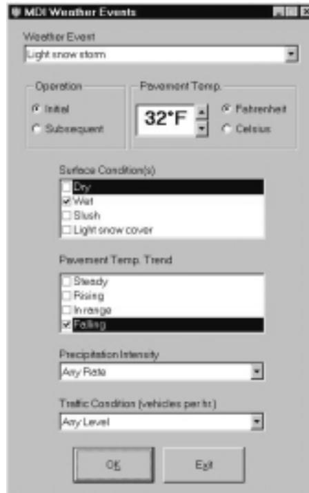
**Figure 43: Materials Distribution Intelligence Configuration GUI**
