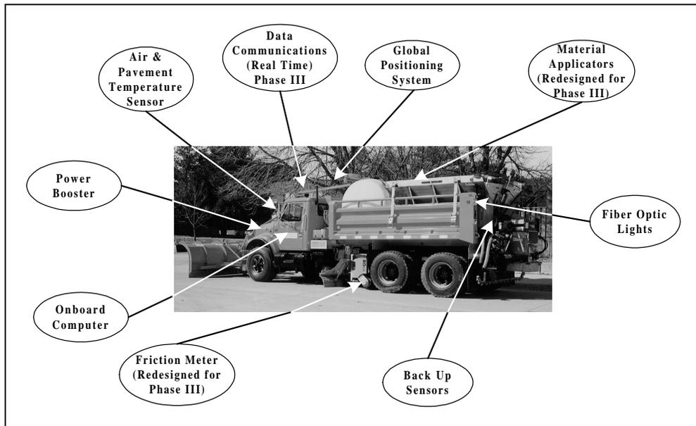
**Figure 2: Phase II Prototype Concept Vehicle Design**
