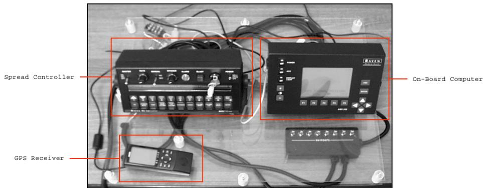
**Figure 38: Mobile System Laboratory Configuration**
