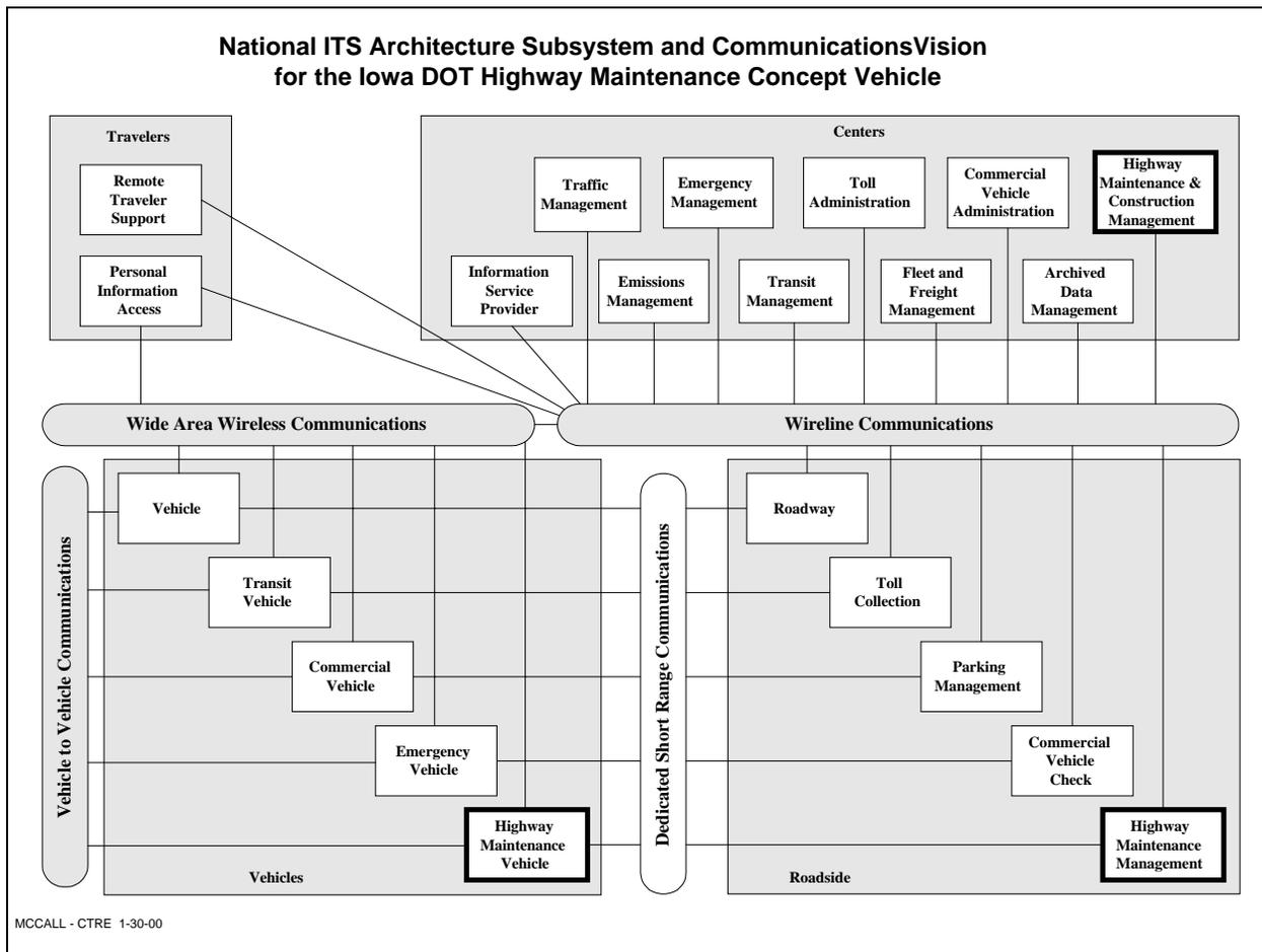
**Figure 5: National ITS Architecture with HMCV Vision**
