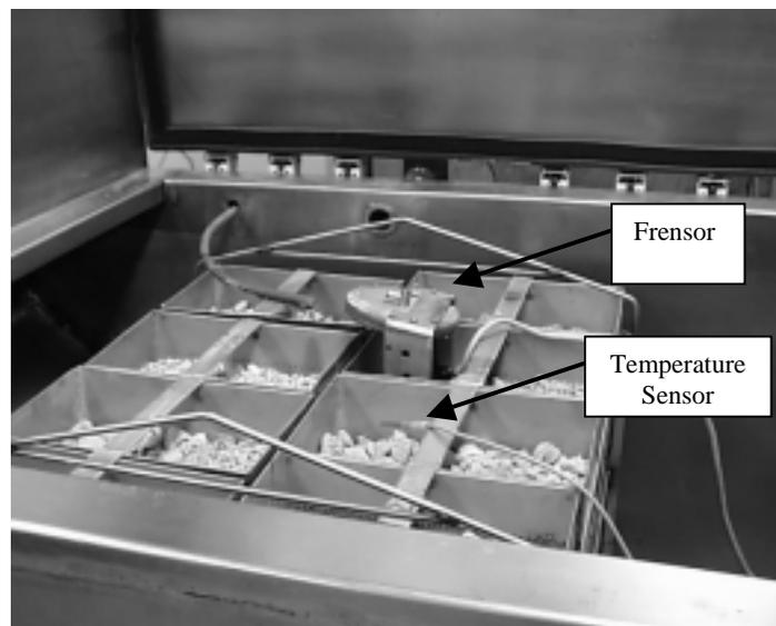
**Figure 26: Frensor sensor placed in freezer**
