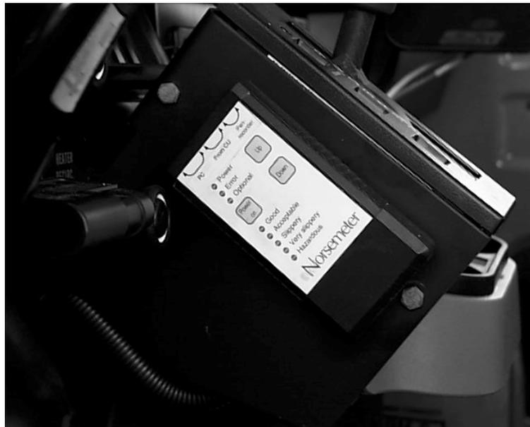
**Figure 13: Operator Panel Installed in Truck**
