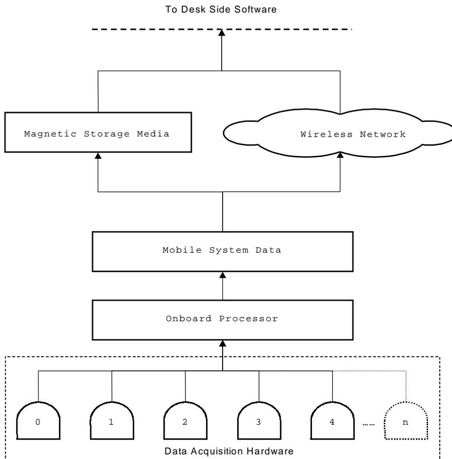
**Figure 35: Mobile System Data – Conceptual Architecture**
