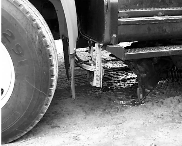
**Figure 20: Frensor device mounted on HMCV**
