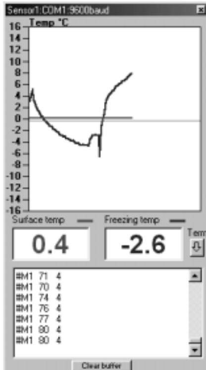
**Figure 31: Graph Data from February 1, 2002 as Recorded on Computer. Taken near MM 95 in Ankeny Iowa RWIS Station**
