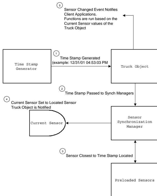
**Figure 37: Sensor Synchronization Process**
