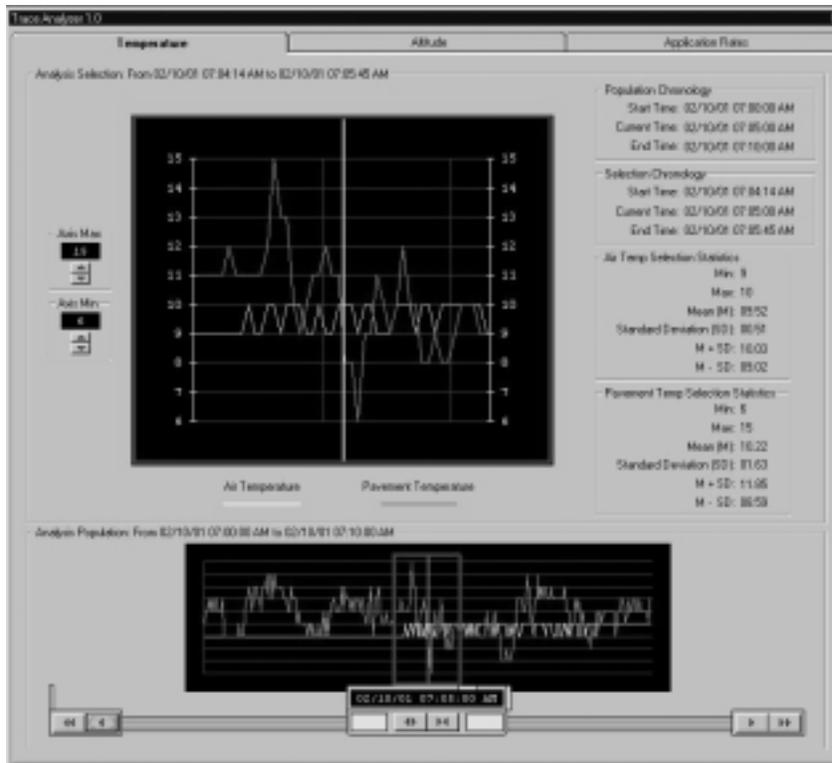
**Figure 44: Thermal Trace Chart Analysis Tool**
