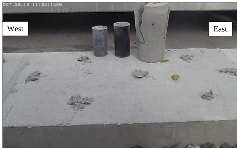
Figure 21. Chemical splitting on day four (after 96 hours)
