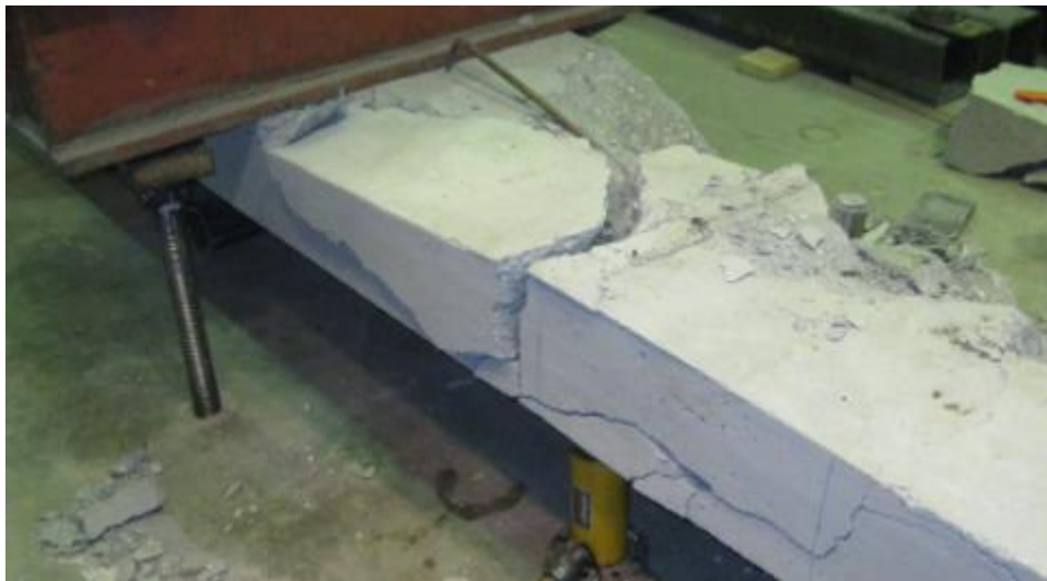
Figure 30. Third peeling test (3 shear studs) (Dang 2013)
