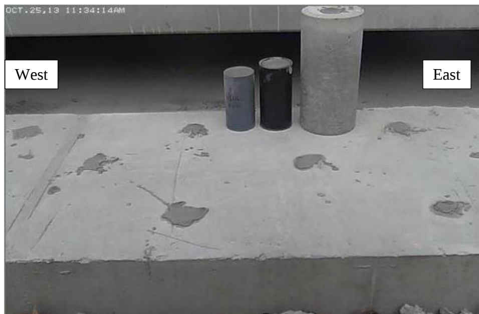
Figure 17. Chemical splitting specimen and the grout
