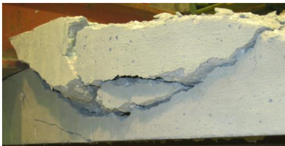
Figure 32. Fifth peeling test (3 shear studs) (Dang 2013)
