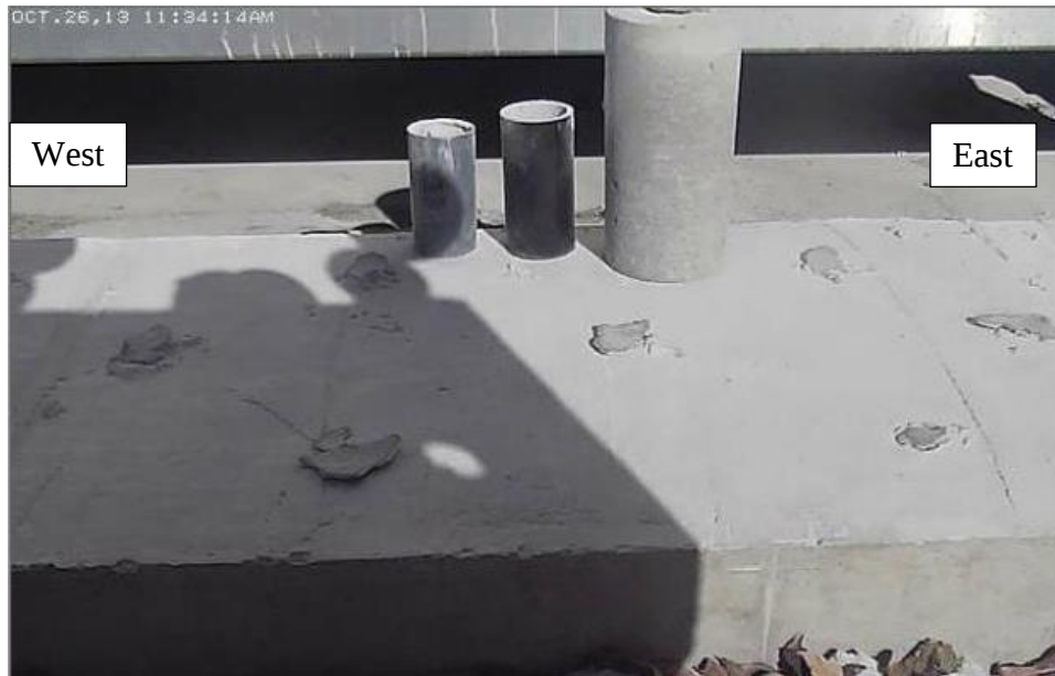
Figure 18. Chemical splitting on day one (after 24 hours)
