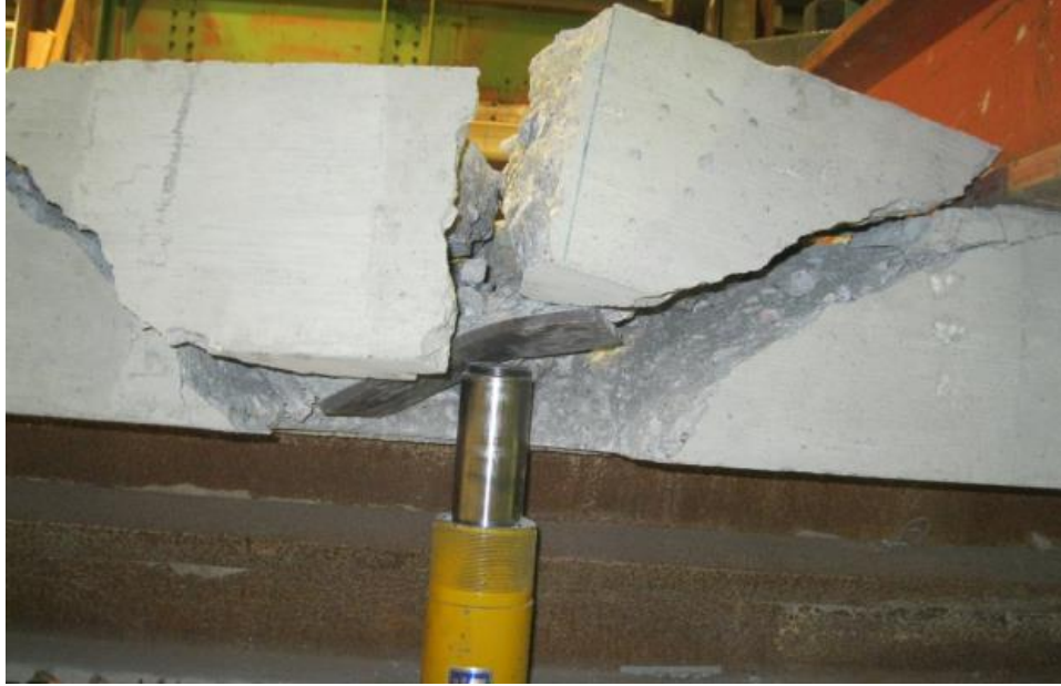
Figure 29. Second peeling test (3 shear studs) (Dang 2013)
