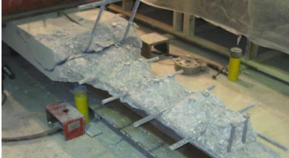
Figure 35. Second peeling test (2 shear studs) (Dahlberg 2014)
