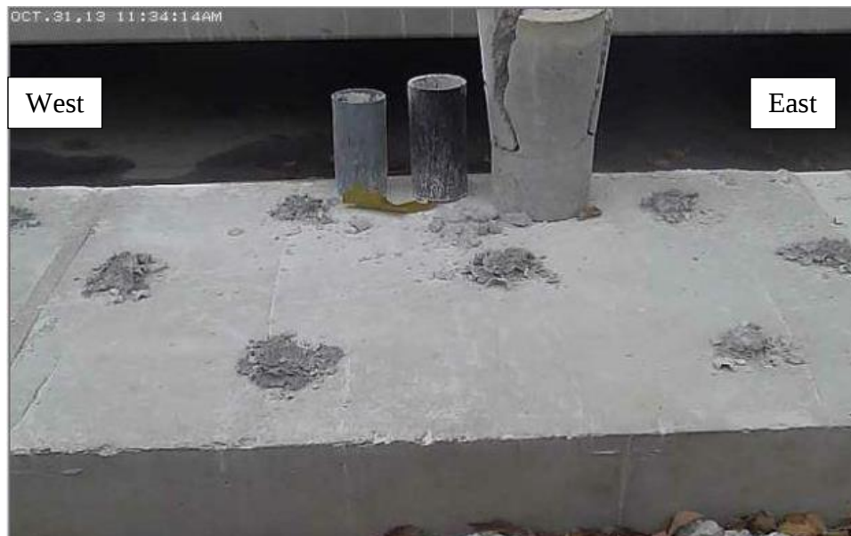
Figure 23. Chemical splitting on day six (after 144 hours)
