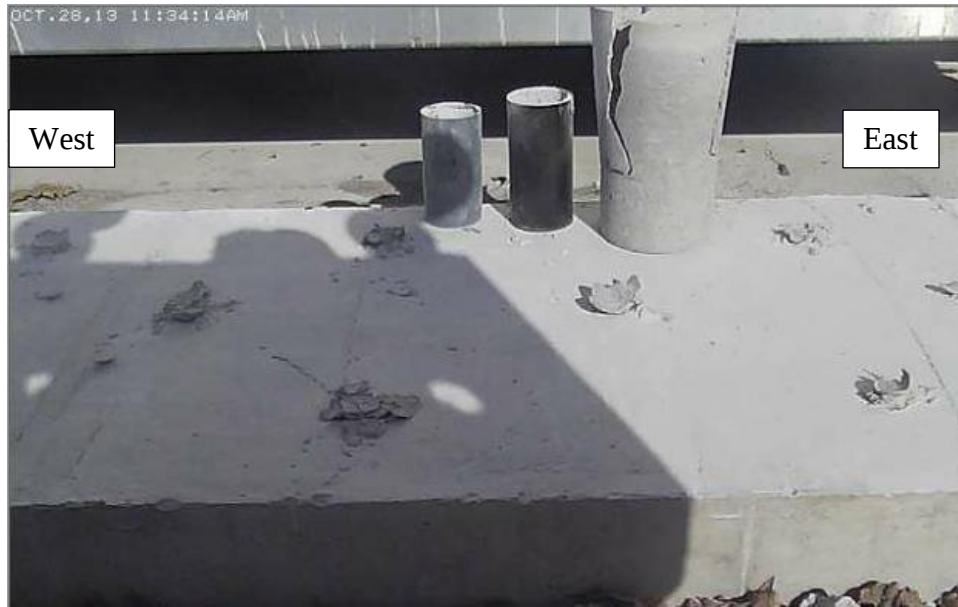
Figure 20. Chemical splitting on day three (after 72 hours)
