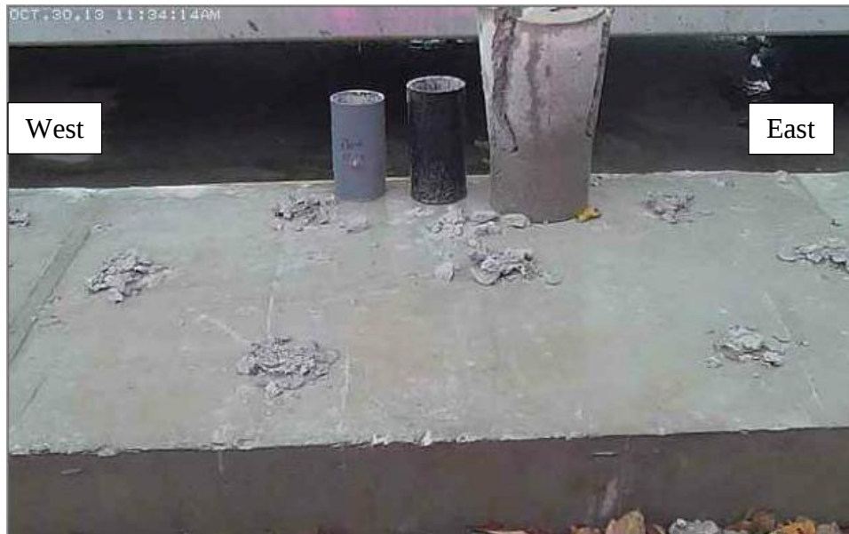
Figure 22. Chemical splitting on day five (after 120 hours)
