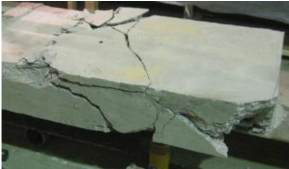
Figure 34. Top view of the first peeling test (2 shear studs) (Dahlberg 2014)
