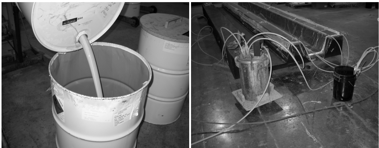
Figure 6. Example of VARTM process
