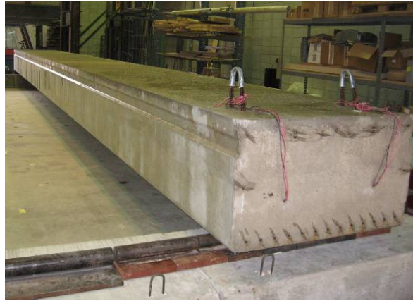
Figure 3.1. Photograph of a precast box girder used for laboratory testing
