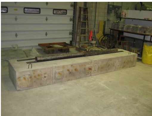
a. abutment and roller placement
