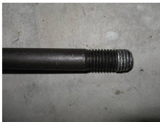
d. bolt with sheared base plate threads
