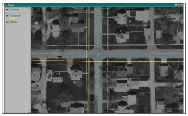
Figure 13. Cartography Alignment Error
