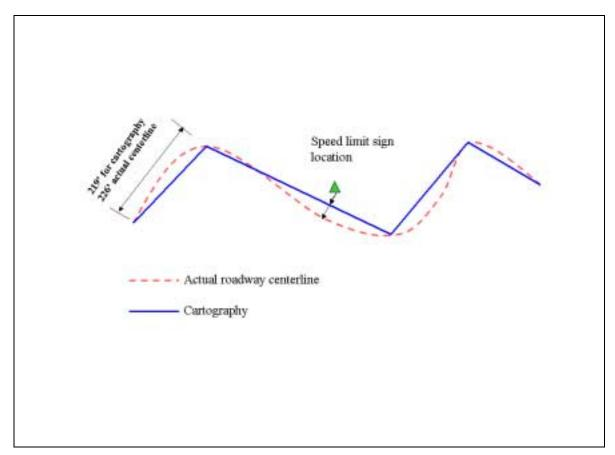
Figure 10. Insufficient Polyline Resolution
