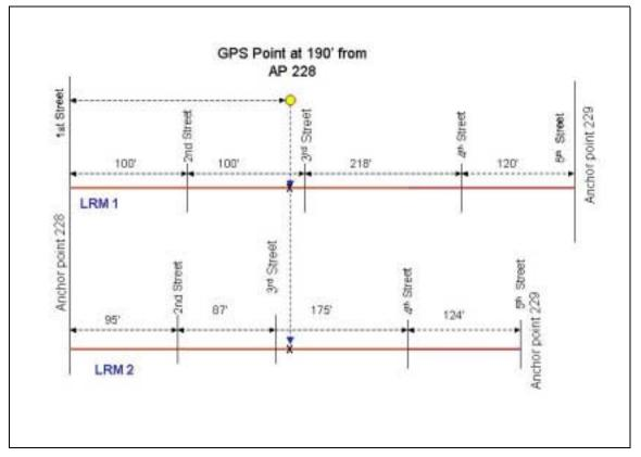
Figure 19. Point Mapping to Different Roadway Segments
