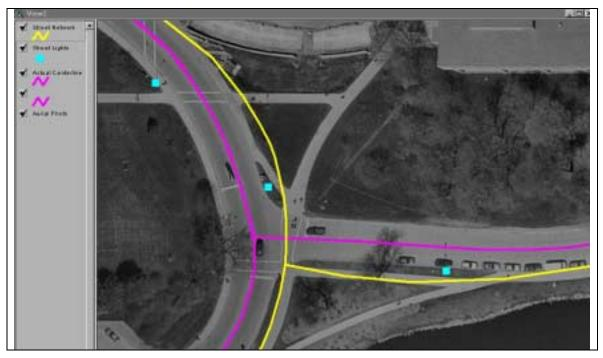
Figure 15. Points Mapped to Wrong Side of Segment (Cartography vs. Centerline)
