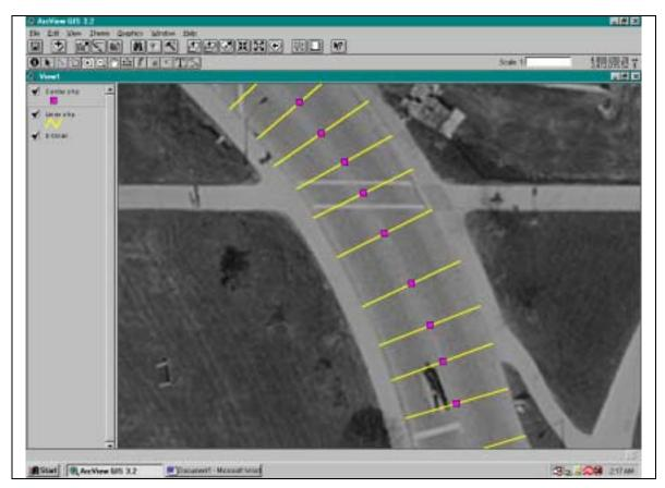
**Figure 6. Centerline Determination**
