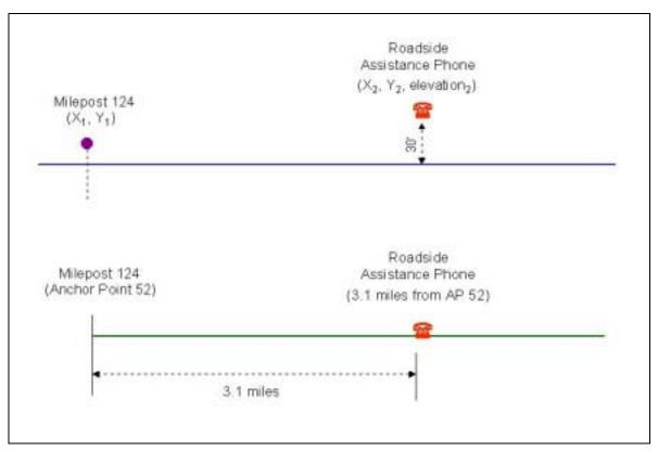
Figure 8. GPS vs. LRS
