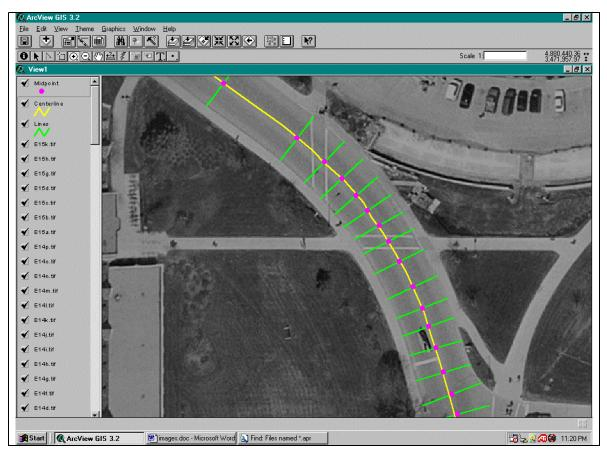
Figure 7. Calculation of Roadway Centerline
