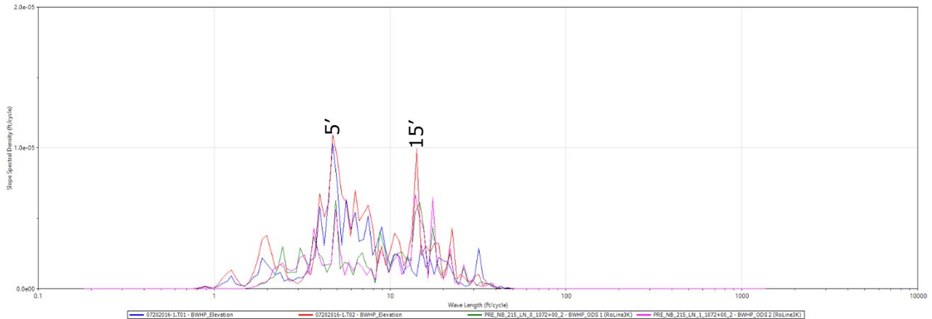
Figure 7. PSD Analysis Showing Joint Spacing at 15' and 5' Harmonic Wavelengths Contributing to Pavement Roughness
