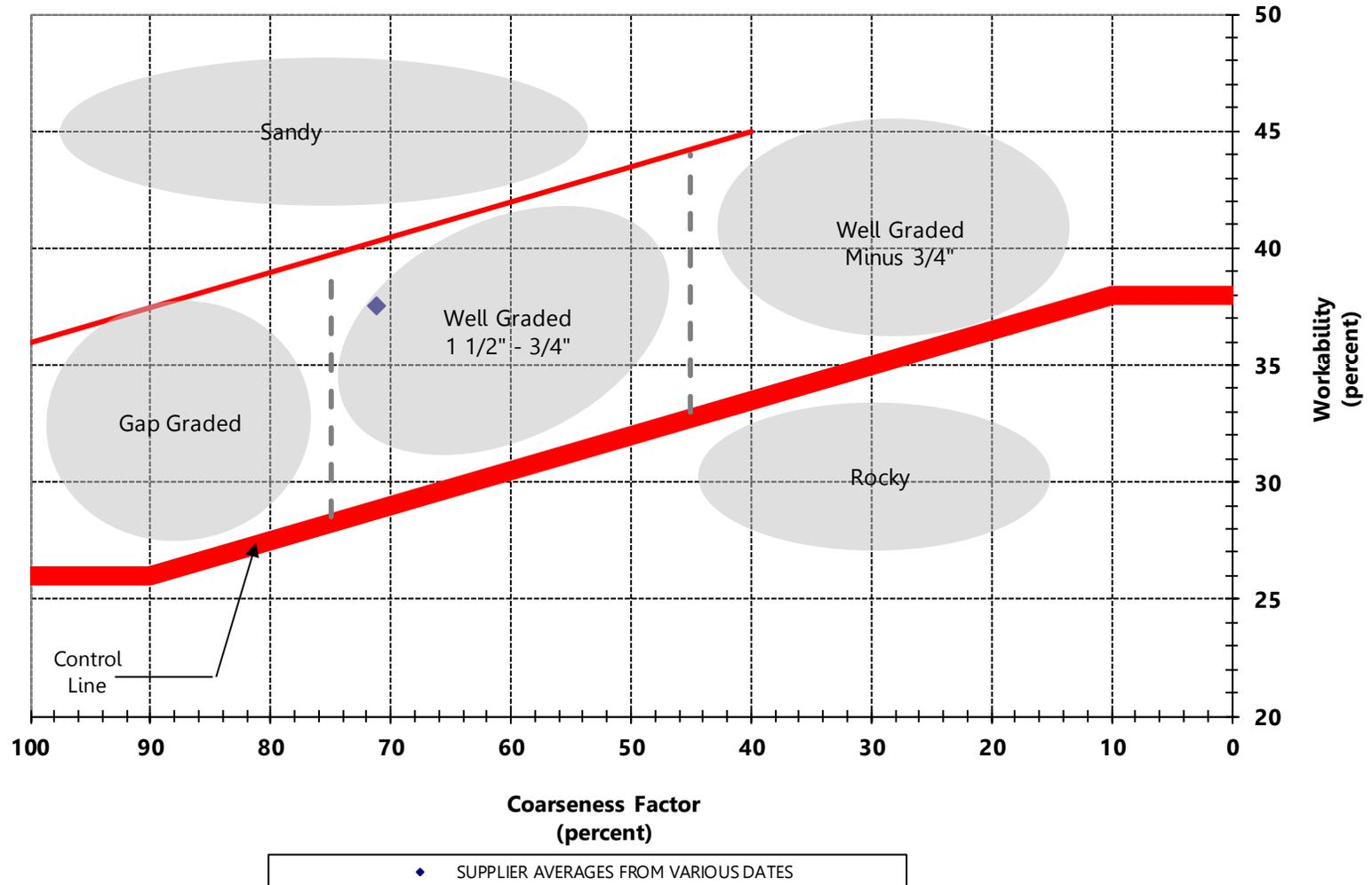
Figure 6. I-215 Combined Gradation Coarseness and Workability Factors
