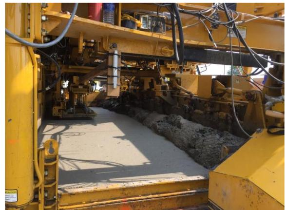
*Figure 4. DBI Section of the Paver Showing the Oscillating Finisher*
