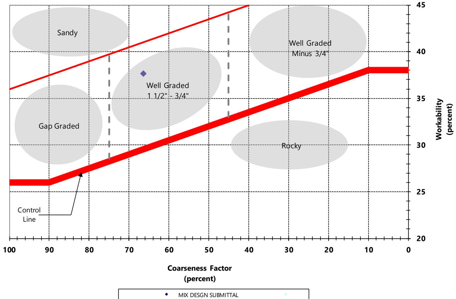
Figure 6. I-69 Combined Gradation Coarseness and Workability Factors
